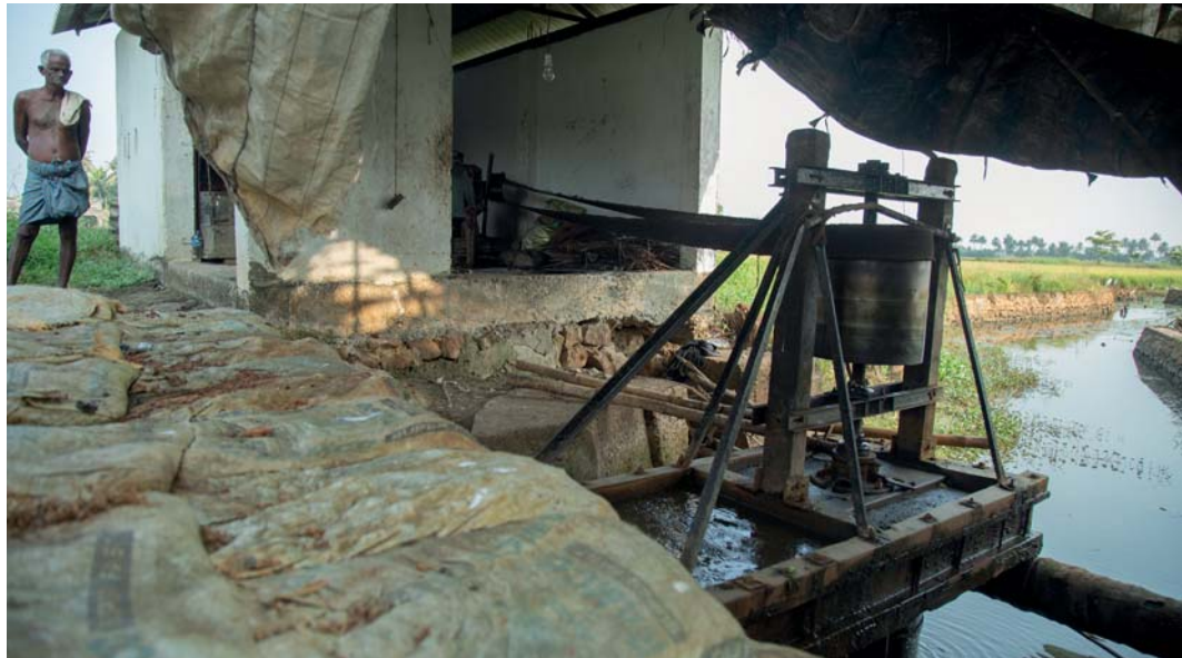
FIGURE 3 The pettium parayum is an indigenous dewatering technology, which runs on electric power, to periodically remove excess water from the paddy fields. (George, 2021)
